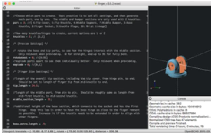
For example, to set `socket_width_bottom` to 28mm, you would change the following line in the file:
